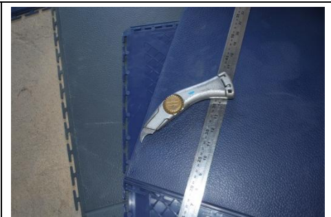
Stanley knife with concave blade
